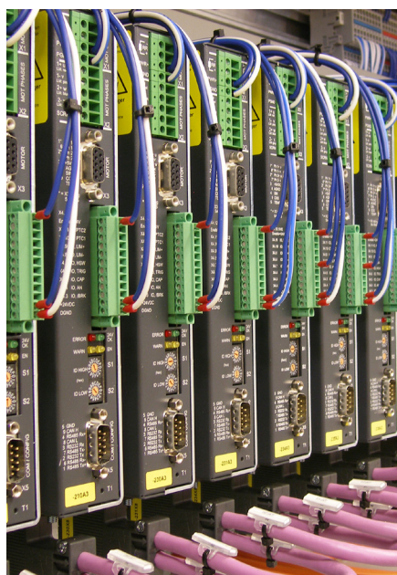
The linear and servomotors on the Z-110 are controlled by particularly compact servocontrollers from LinMot, with a PROFIBUS interface (DP) and 15A maximum current. (Photo: Zellwag)
